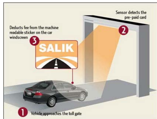
Figure 1. Salik toll gate system procedure [12].
