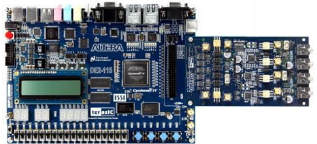
Fig. 5. DE2-115 equipped with the Terasic Data Conversion HSMC Card
