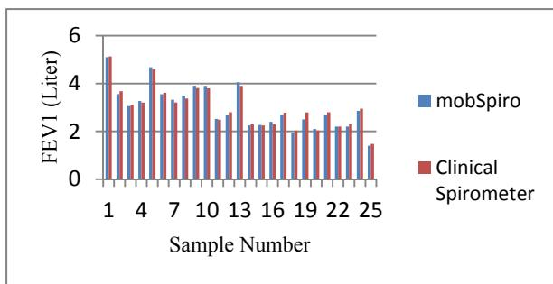
**Figure 5. FEV1 differences between clinical spirometer result and MobSpiro result.**
