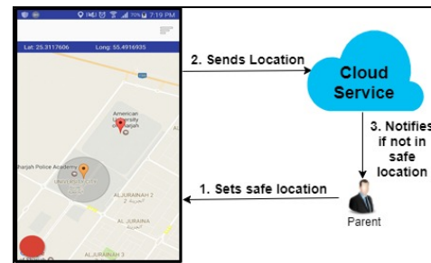
Fig. 16. Conceptual Implementation View of the Monitoring System
