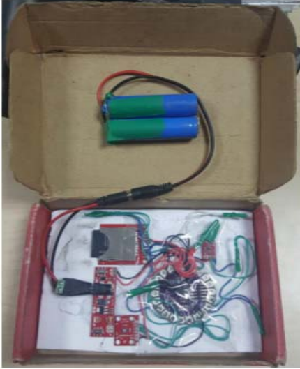
Fig 2. Sensor box to collect accelerometer and gyroscopic sensor data
