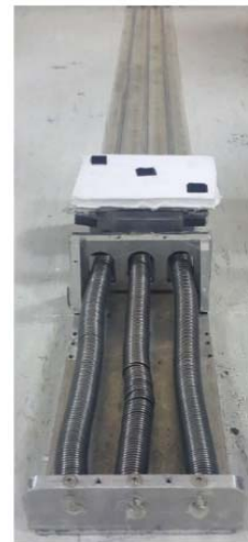
Fig 1. Apparatus to simulate the 40g crash
