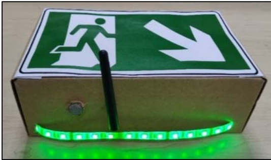
Fig. 4. Smart exit sign including the ESP32 microcontroller, LED strip, WiFi and DigiMesh network.
