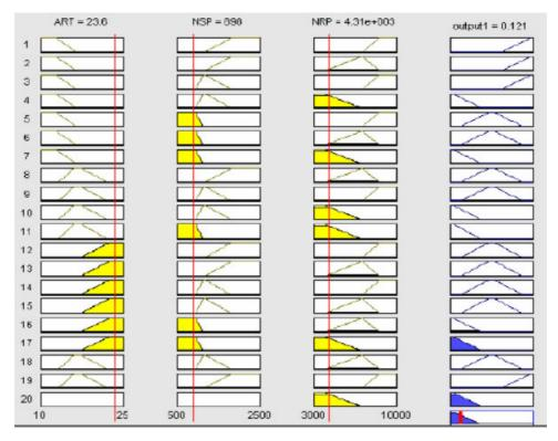
Fig. 5. The Fuzzy Logic rules used to detect port scanning. The inputs to the system are ART, NSP, and NRP.
